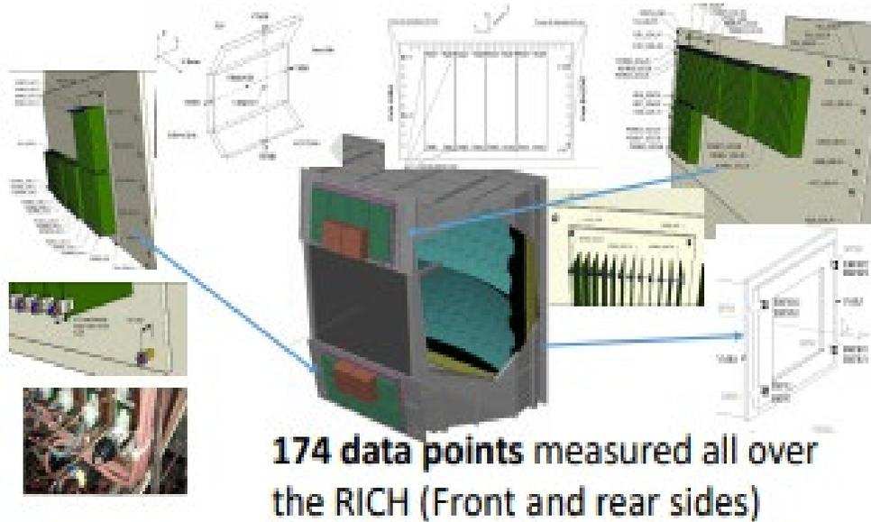
**3 survey campaigns. 174 data points collected all over the RICH surface. Data points have stability in different years within 1 mm . Suggested data and CAD drawing Consistency within 1 mm. Survey precision is 0.5 mm**
