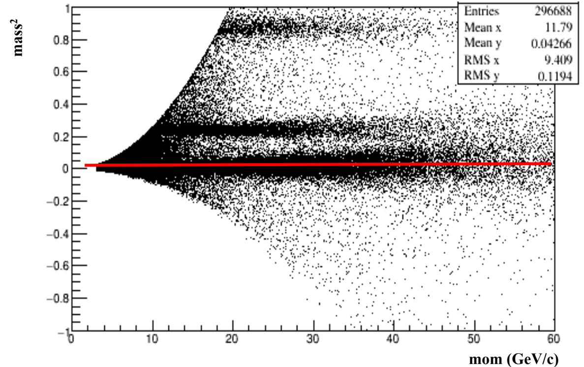
Refractive index NOT rightly set (electron contamination present)
