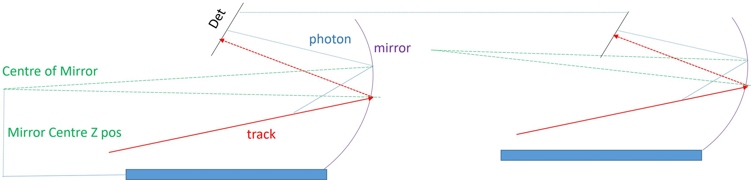
The Z position of the mirror has opposite effect of the detector Z position!
