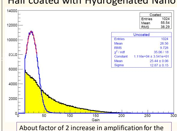
Voltage Stability has decreased. Frequent sparks have been observed. Can not reach nominal voltage obtained before coating.
