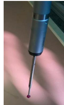
Mitutoyo EURO CA776 coordinate measuring machine with ruby touch probe, hosted in a thermalized room
