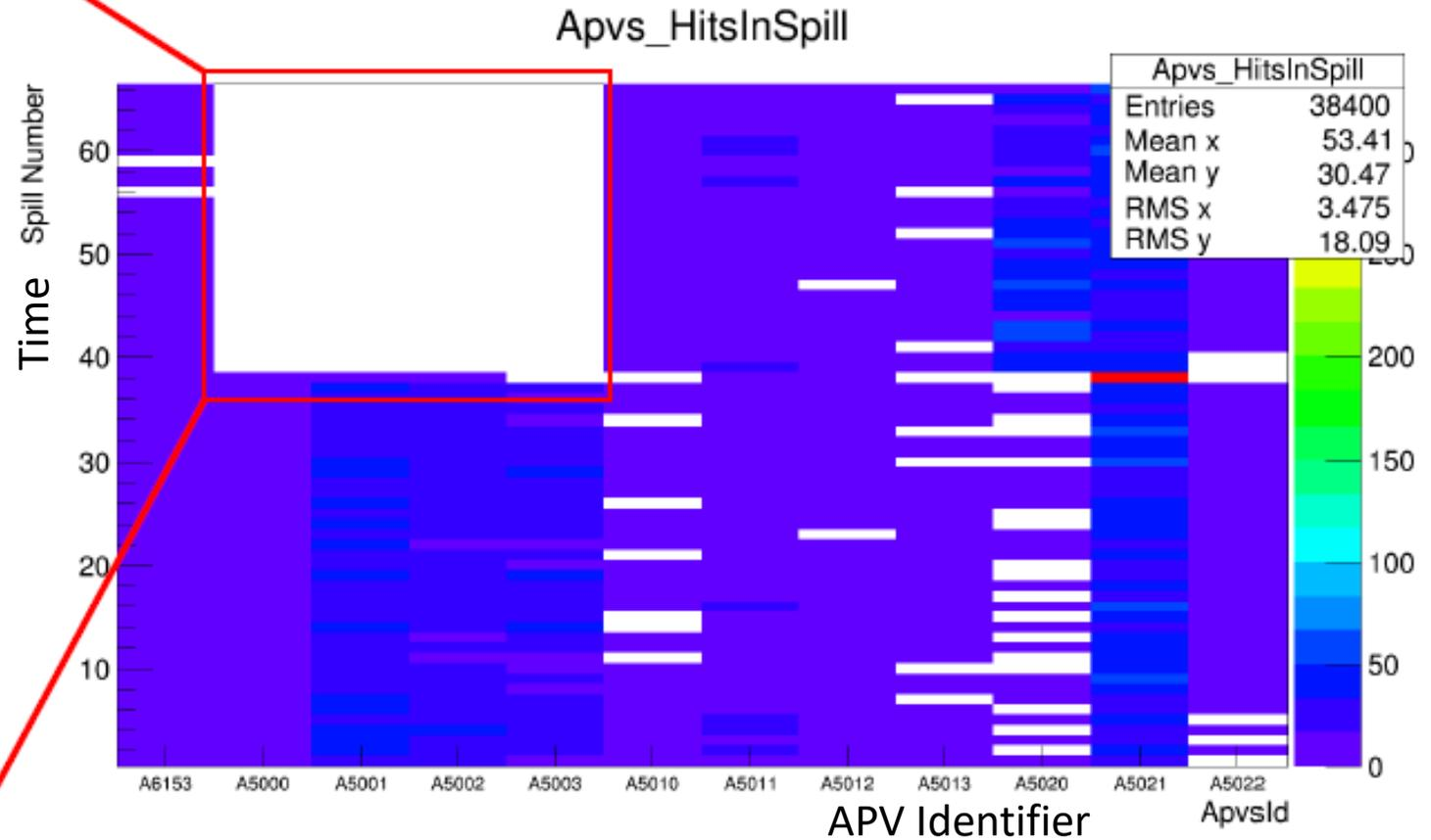
A log has been created with SrcId spill no. and no. of missing/notworking APVs
