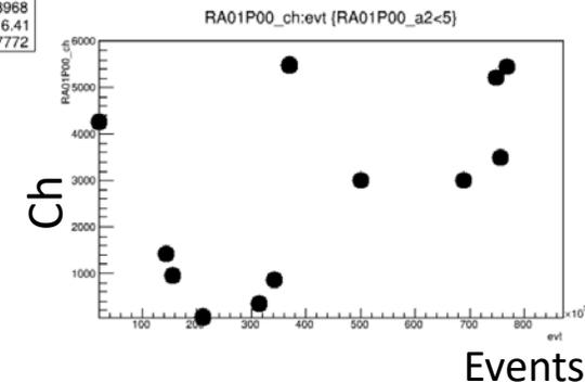
The tiny 'Readout Error' is not localized over events
